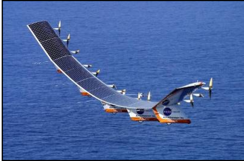
Helios wing dihedral on takeoff
